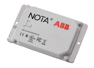
NOTA® Smart Sensor converts traditional pumps into smart, wirelessly connected devices. It enables you to monitor the health of your pumps, identify inefficiencies and improve reliability and safety.
